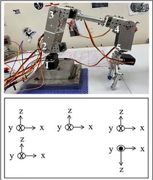
Figure 12. Coordinate system of the robotic arm.
