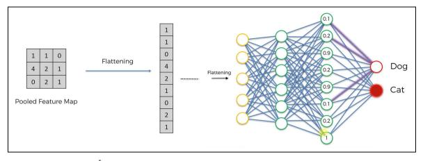
Figure 4. Fully connected layer.<sup>5</sup>
